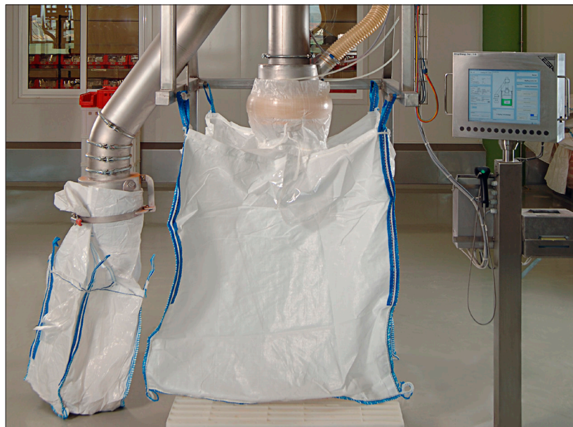
At „Almi“ IFS compliant metal detection is performed directly before filling of the spice products in bigbags.
